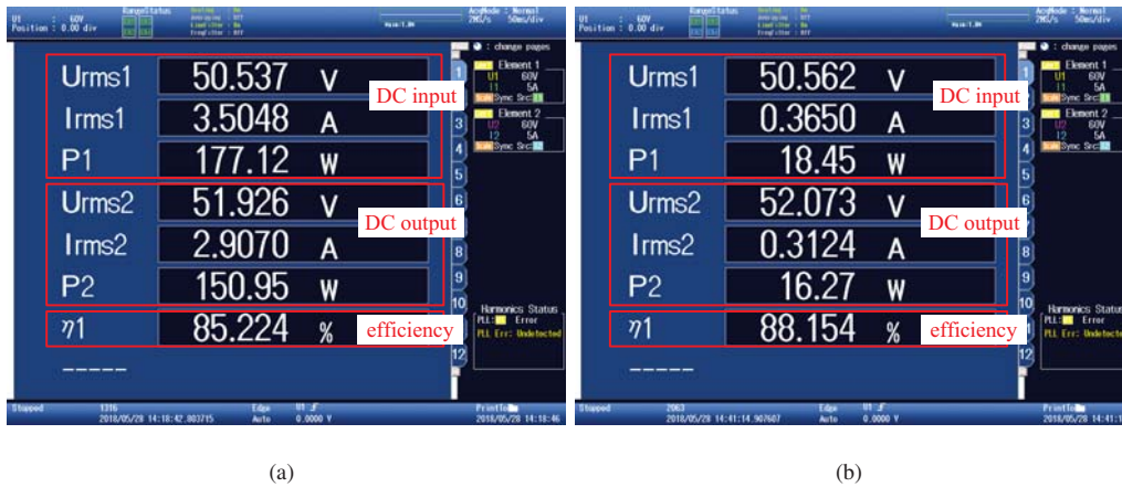
Fig. 15. Screen capture of efficiency measurement at (a) the start and (b) the end of CV charging.
